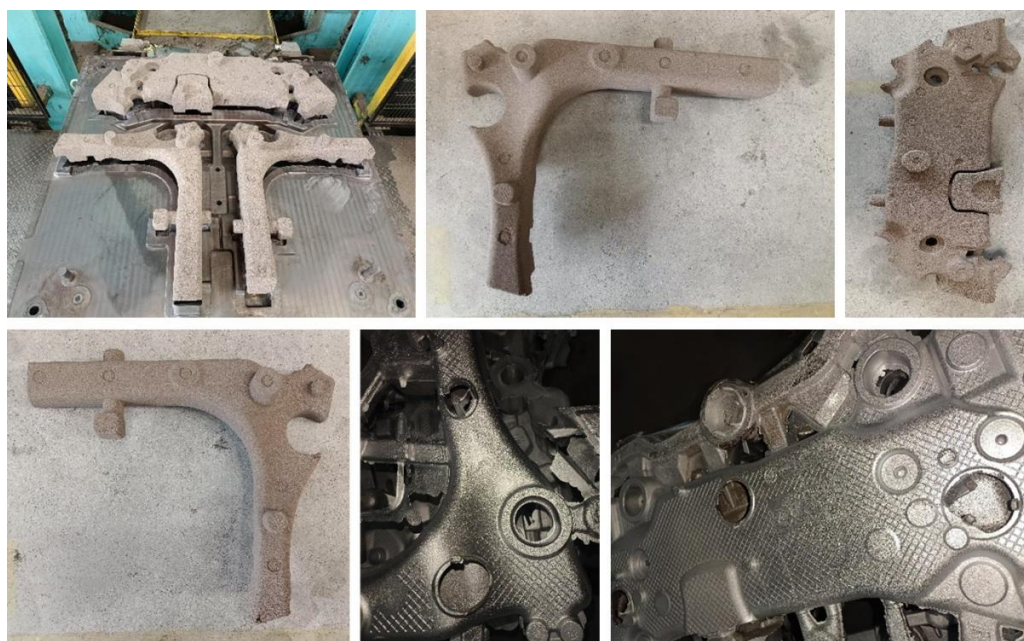
Fig. 5: Improved quality of sub-frame core and casting by SQ binder
