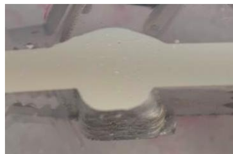
Fig. 4: MIG-weld seam No. 3.1 (Castaduct-42)
