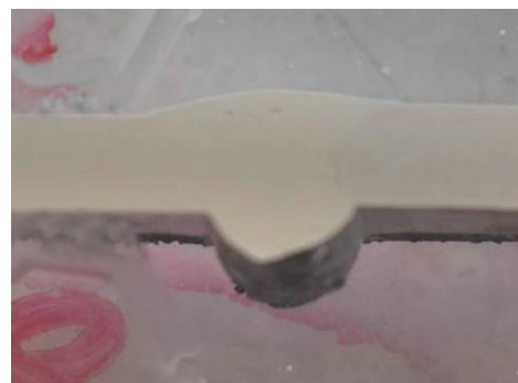
Fig. 6: MIG-weld seam No. 4.1 (Magsimal-plus)
