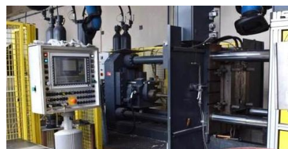
Fig. 2: High pressure die casting cell in the Tech Center Rheinfelden
