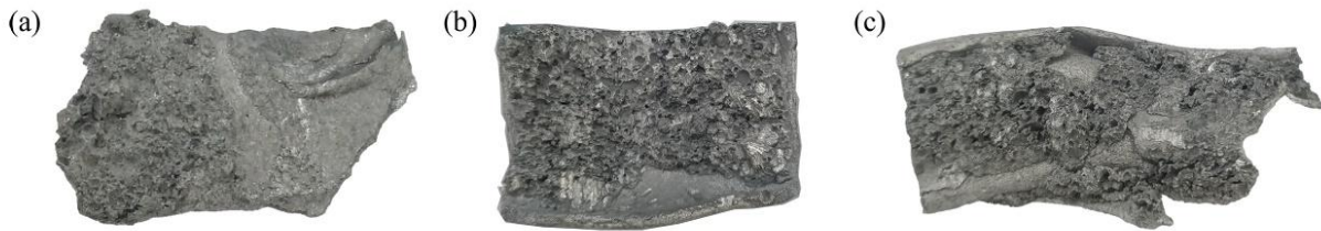
Figure 6 Interface morphology between aluminum foam core and aluminum alloy tubes after IFAFSDTs were separated: (a) inner tube; (b)(c) outer tube.
