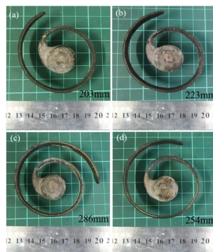
Fig. 4 Test results of flow properties of alloys with different C content (a) 0.02%C (b) 0.04%C (c) 0.06%C (d) 0.08%C
