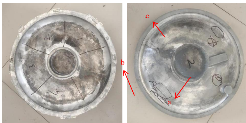
Figure 3. Finished drawing of ZM5 partition component and marking of sampling positions
