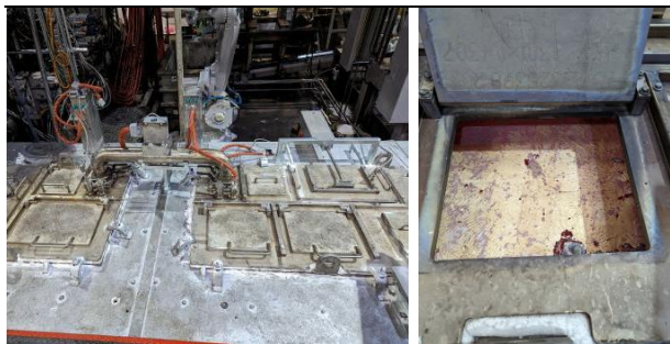
Fig. 1. Casting Line with a Melting Capacity of 1.400 kg Mg/h & ASKI inert gas supply
