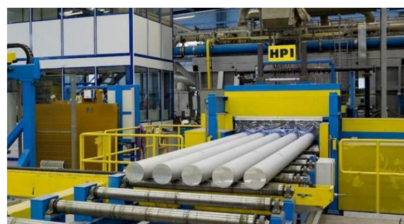
Fig. 3. HPI ForgeMaster Line for the production of Magnesium billets or ingots
