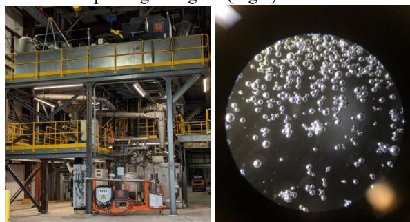
Fig. 2. Novel Atomizer developed @ GGG for the production of globular particles 0.2 - 1.0 mm
