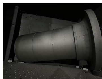
Fig. 9 : Condition of the wind power main shaft after shot blasting
